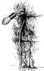
Fig. 23.—Method of Arranging Glow Lamps to the Walls of the House Tower.
